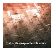
plastic tiles. The mesh, made from periodically repeating, sinusoidal polypropylene fibers, provides in-plane elasticity and holds the scales, made from cellulose acetate butyrate, in place as the material is deformed. It also provides a mechanism for scales to rotate and interact with adjacent scales. The mechanical response during in-plane deformation, flexure, and indentation showed many of the advantageous attributes of its biological counterpart. - MSL
