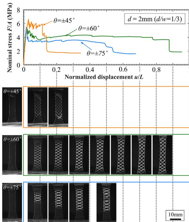
**Fig. 6.** Tensile response and associated deformation mechanisms for cross-ply-architected glasses with  $\theta = 75^\circ$ ,  $60^\circ$  and  $45^\circ$ . For all configurations  $d = 2$  mm (corresponding to  $d/w = 1/3$ ).
