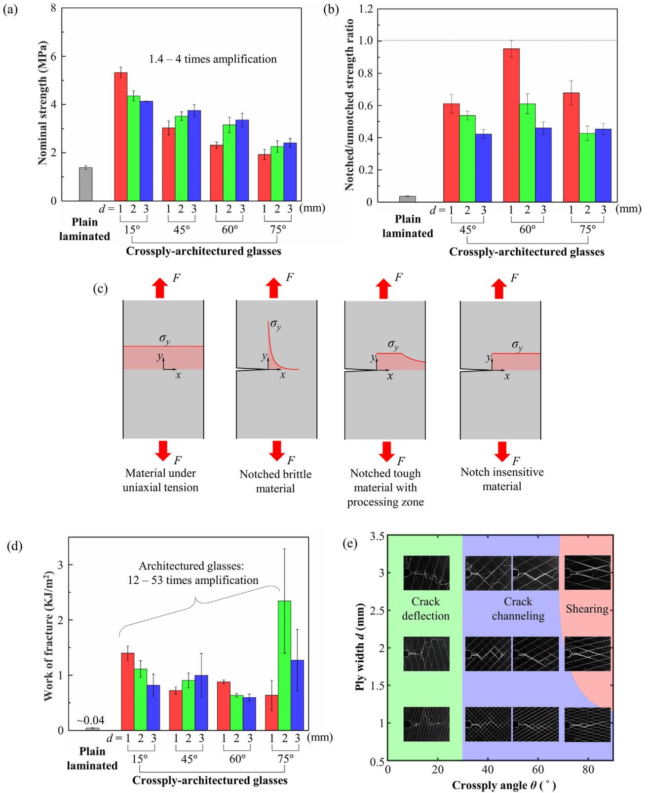
**Fig. 12.** (a) Nominal strength of the notched samples for different configurations; (b) Ratio of notched and unnotched strength (a ratio of 1 means that the material is notch insensitive); (c) Illustration showing how tough and deformable materials redistribute stresses at a notch; (d) Work of fracture for different laminated glass designs; (e) Failure mode map as function of ply angle  $\theta$  and ply width  $d$ .
