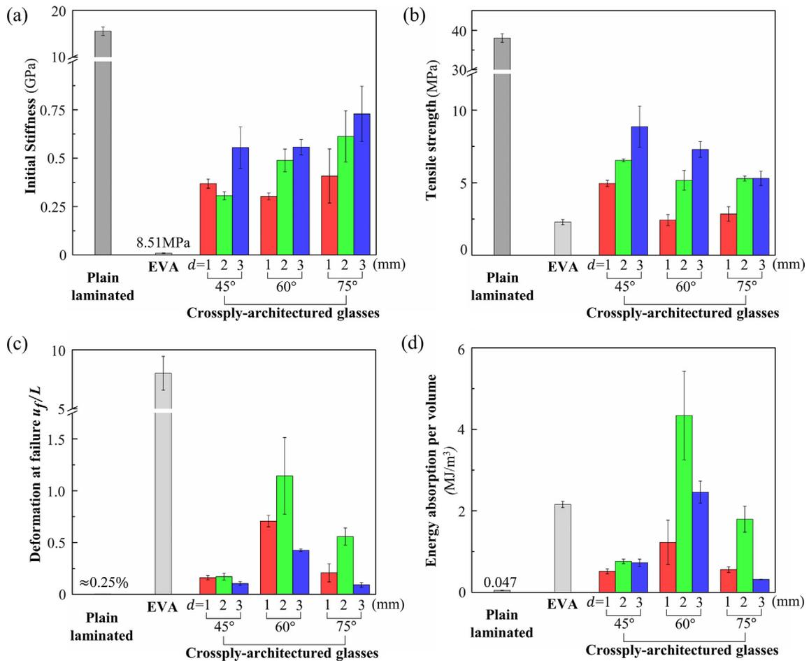
**Fig. 8.** Tensile properties for plain laminated glass, pure EVA and architected cross-ply glasses: (a) Initial stiffness; (b) tensile strength; (c) deformation at failure and (d) energy absorption based on the failure criterion that the nominal stress drops below the yielding strength of EVA.
