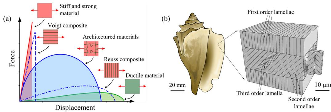
**Fig. 1.** (a) Generic force displacement curve for a stiff and strong (but brittle) material, a low-strength ductile material, and for three possible composites of these materials; (b) Cross-ply architectures in conch shell.
