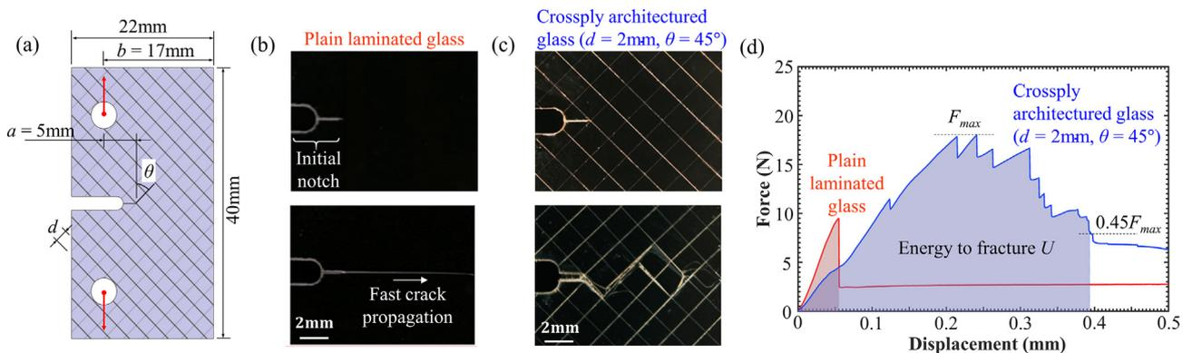
**Fig. 11.** (a) Dimensions of fracture test samples; (b) Straight and rapid crack propagation in plain laminated glass; (c) progressive and twisted crack propagation in cross-ply architected glass; (d) typical tensile notched force-displacement curves for plain laminated glass and for cross-ply architected glass.
