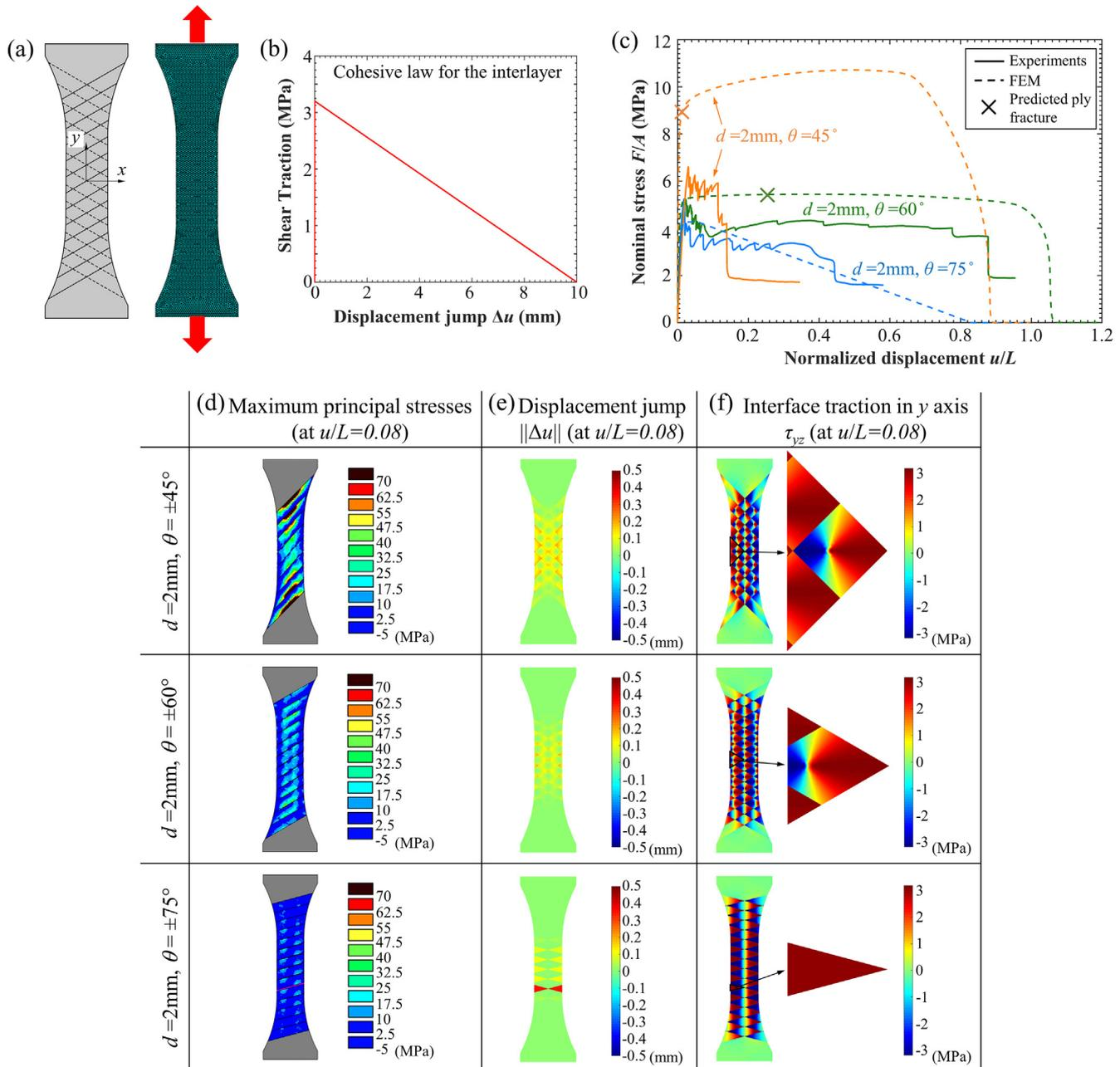
**Fig. 9.** (a) Finite element model setup; (b) Cohesive law simulating the shear response of the EVA interlayer; (c) Experimental and finite elements force-displacement; (d) Maximum first principal stresses in the plies; (e) Displacement jump  $\Delta u$  across the layers and (f) distribution of shear tractions at the interlayer.
