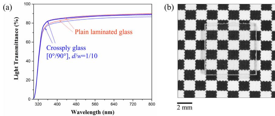
**Fig. 4.** Optical properties of the plain and architected laminated glasses: (a) light transmittance and (b) optical clarity: No decrease in light transmittance, image distortion or decrease in the appearance of objects was observed for the architected materials.
