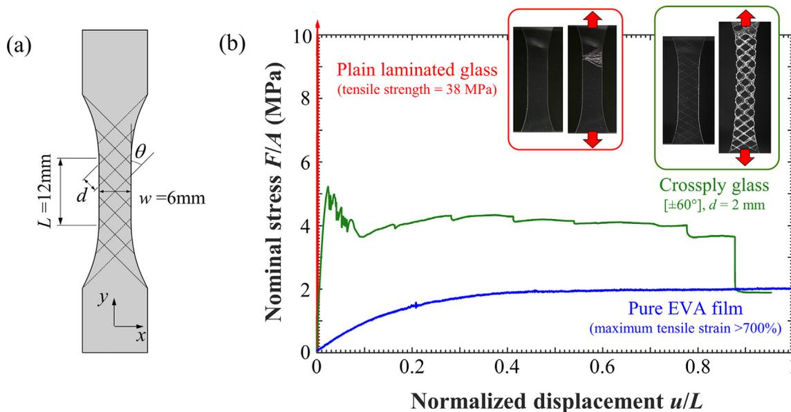
**Fig. 5.** (a) Overview of tensile test samples; (b) typical tensile responses for pure EVA, traditional laminated glass and cross-ply architected glass.
