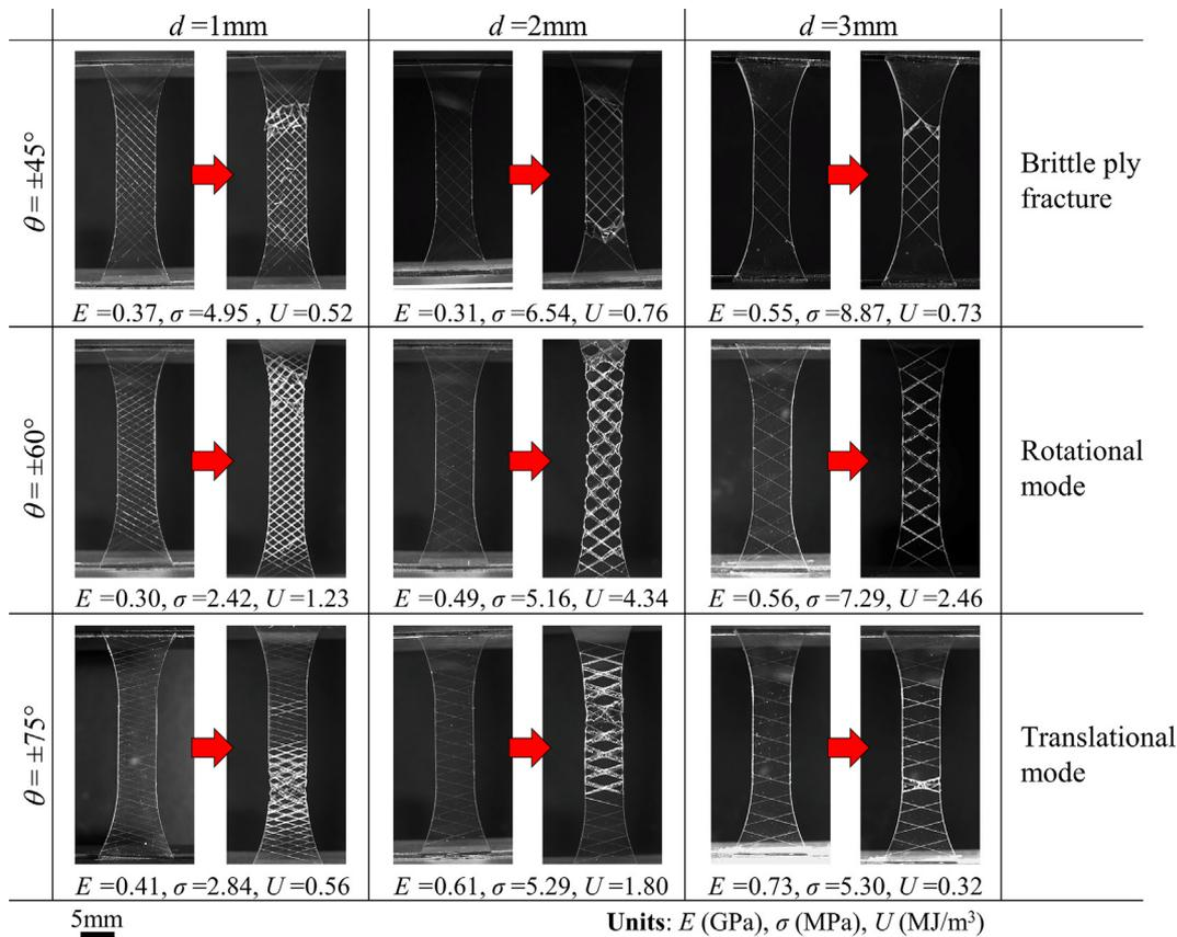
Fig. 7. Deformation map showing three tensile deformation and failure modes for cross-ply architected glasses as function of ply angle and ply width, supplied with stiffness  $E$ , strength  $\sigma$ , and unit volume energy absorption  $U$  for each configuration.
