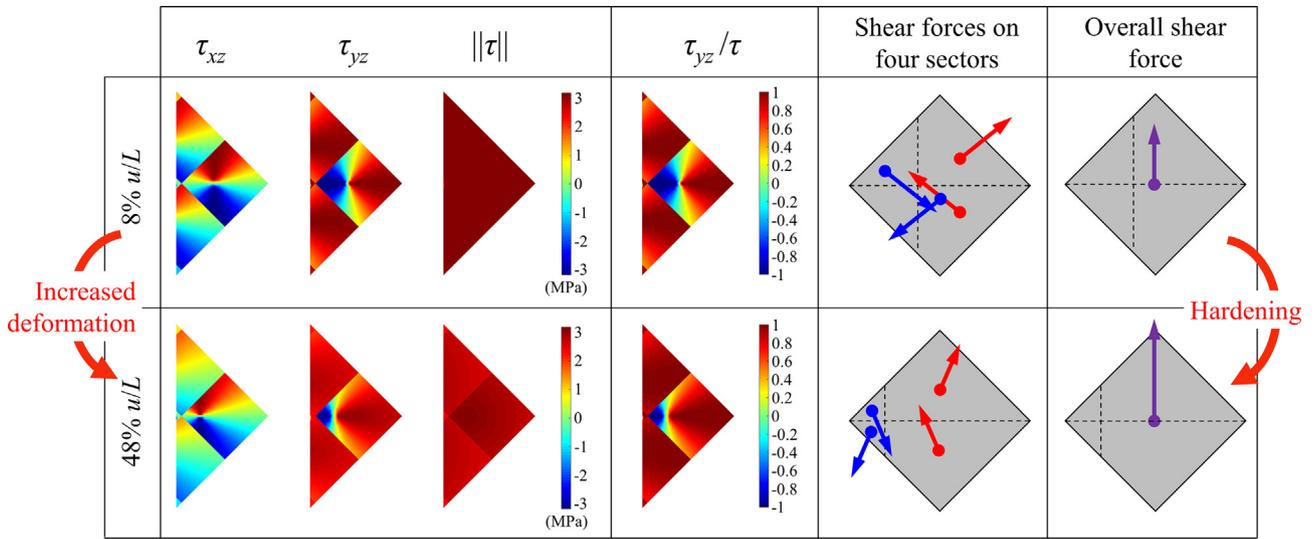
**Fig. 10.** Local shear stresses  $\tau_{xz}$ ,  $\tau_{yz}$ , magnitude of shear stress  $\tau$ , distribution of  $\tau_{yz}/\tau$ , schematic showing the change of magnitude and direction of force vectors on four different sectors at the interlayer and resulting overall force. Each data is given at two level of deformation in post yield regime. These results demonstrate how global strain hardening can be attained from a softening interface.
